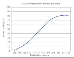
The efficiency chart above is extrapolated from particle size versus efficiency information when evaluated per
