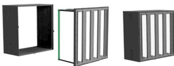
A V-Bank filter is the optimum air filter configuration for energy savings. In installations limited to front-load only and no room downstream of the holding frame, an optional and reusable ES<sup>3</sup> Box Kit is available. The box kit mounts permanently to the upstream side of the frame and the Durafil ES<sup>3</sup> is installed to create a box-style filter.
