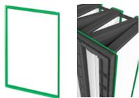
For those critical applications that require additional protection against bypass, an optional 360° Gasket is available. The gasket installs around the entire perimeter of the Durafil ES<sup>3</sup> and seals tight against holding frames. Unique corner shape limits wrinkles from developing once the filter is fastened firmly in place.
